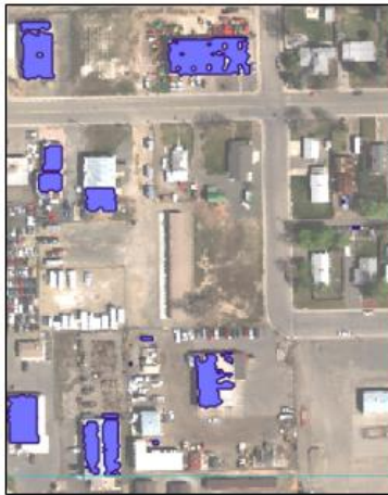
Figure 18: Shapefile of SAM target detection results for galvanized roofing, displayed over the source image.
