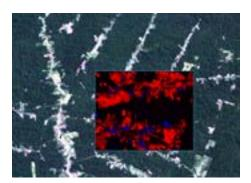
THIS IMAGE PREVIEWS ENVI CHANGE DETECTION RESULTS. USING TWO LANDSAT IMAGES TAKEN AT DIFFERENT TIMES, ENVI AUTOMATICALLY IDENTIFIED DEFORESTED AREAS (IN RED). THE BLUE AREAS INDICATE NEW GROWTH OR PLANTING.
