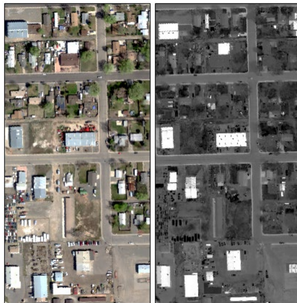
Figure 16: NEON hyperspectral image (left) and OSP rule image with Gaussian display stretch applied (right). The target is galvanized metal roofing.
