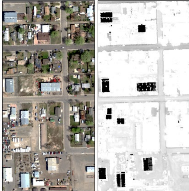
Figure 17: NEON hyperspectral image (left) and SAM rule image with logarithmic display stretch applied (right). The target is galvanized metal roofing.
