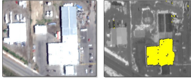
Figure 24: NEON hyperspectral true-color image (left) and SAM rule image with threshold applied (right).
