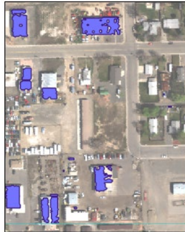
Figure 25: Shapefile of SAM target detection results for galvanized roofing, displayed over the source image.
