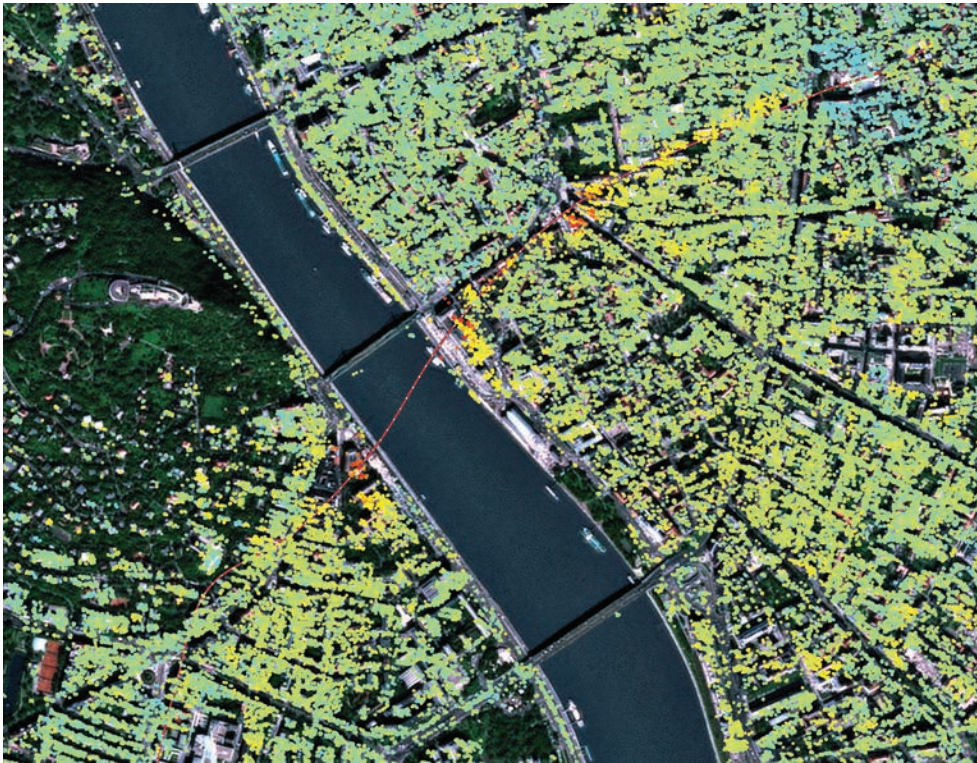
Average displacement rate (color scale between -7 and +7 mm/year), of an area in the city of Budapest, related to the excavation of a new metro station. ©TerraSAR-X data: DLR - Astrium GEO; processing: Astrium GEO.
