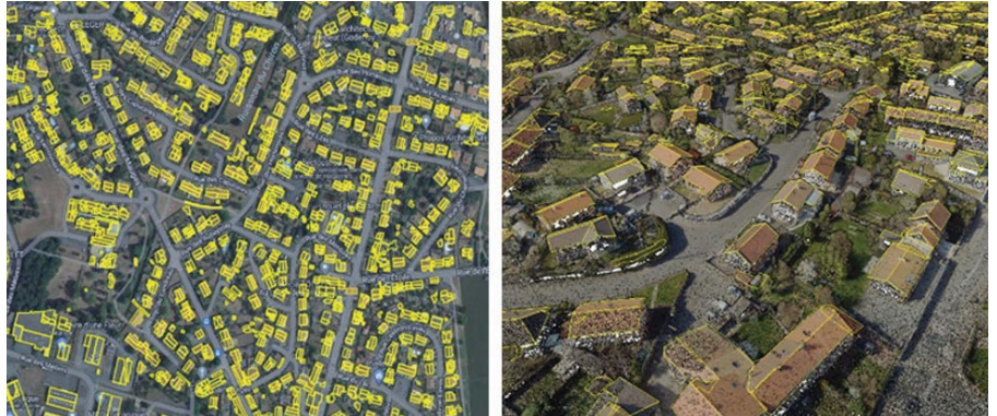
Detected buildings roofs in 2D over Google imagery (left). Detected buildings roofs in 3D over airborne LiDAR (right).
