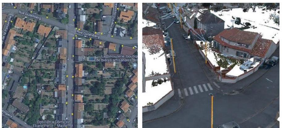
Detected poles in 2D over Google imagery (left). Detected poles in 3D over high-density terrestrial LiDAR with RGB (right).
