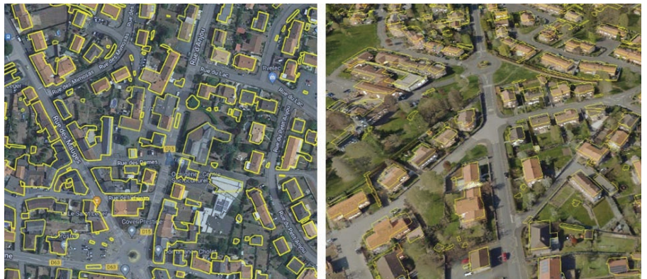
Detected building perimeters in 2D over Google imagery (left). Detected building's perimeters in 3D over airborne LiDAR (right).
