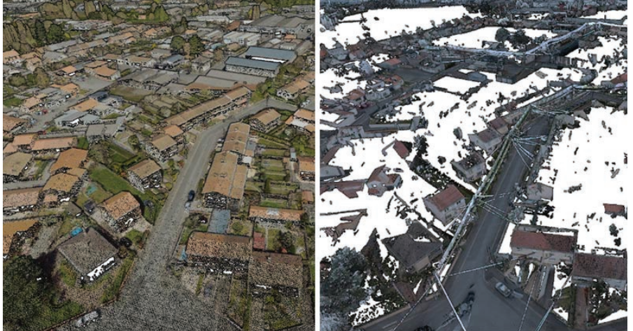
Low density urban airplane Lidar (left). High-density RGB urban mobile LiDAR on the same area (right).
