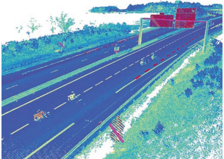
Detected traffic signs in 3D over terrestrial LiDAR with intensity gradient colors.
