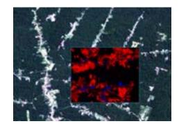
This image previews ENVI change detection results. Using two Landsat images taken at different times, ENVI automatically identified deforested areas (in red). The blue areas indicate new growth or planting.
