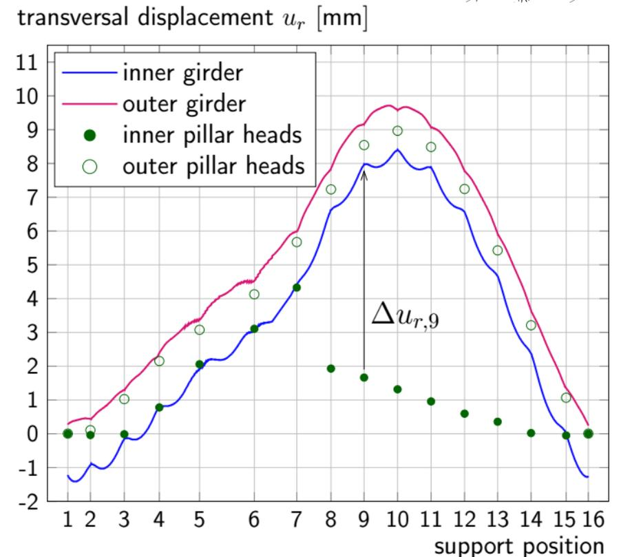
Longitudinal and transversal displacements of the deck and the pillar heads at all support positions under the combination of dead load, prestressing and total temperature increment  $\Delta T=30$  K; the unified coefficient of friction is set to  $\mu=0.05$
