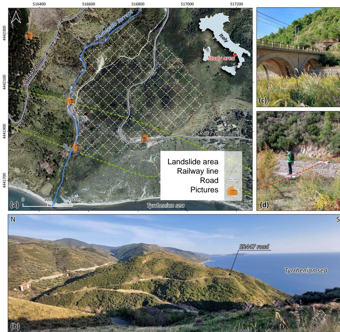
The landslide extends approximately 0.2 km<sup>2</sup> and moves at a rate of about 100 cm/y towards the Fiumicello riverbed. The landslide movements affect the SR447 road and the national railway. Currently, the assessment of the present-day activity and kinematics of the Pisciotta landslide has not been provided yet.
