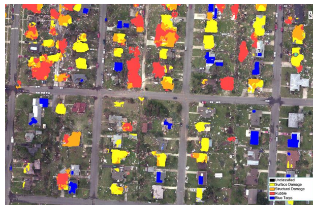
Assess building damage after hurricanes and tornadoes
