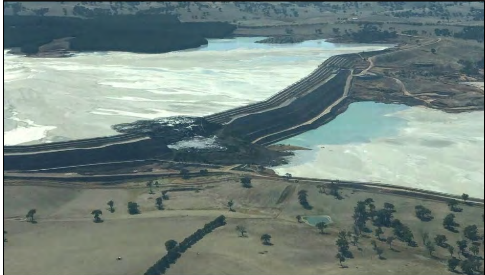
An aerial image showing the collapsed section of the tailings dam. Photo: Supplied
