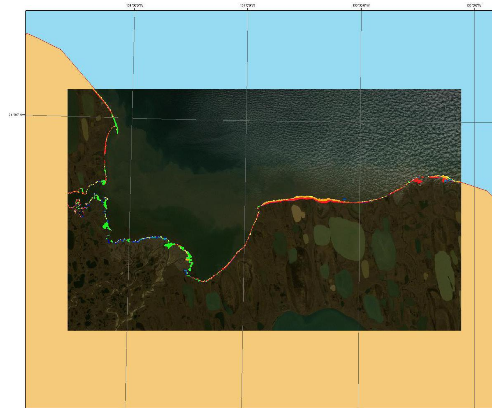
Figure 2 Detailed view of Drew Point and analysis results. Yellow areas are erosional losses from 1974 to 1978, orange from 1978 to 1999, red from 1999 to 2008. Dark blue areas are deposition from 1974 to 1978, light blue from 1978 to 1999, green from 1974 to 2008.
