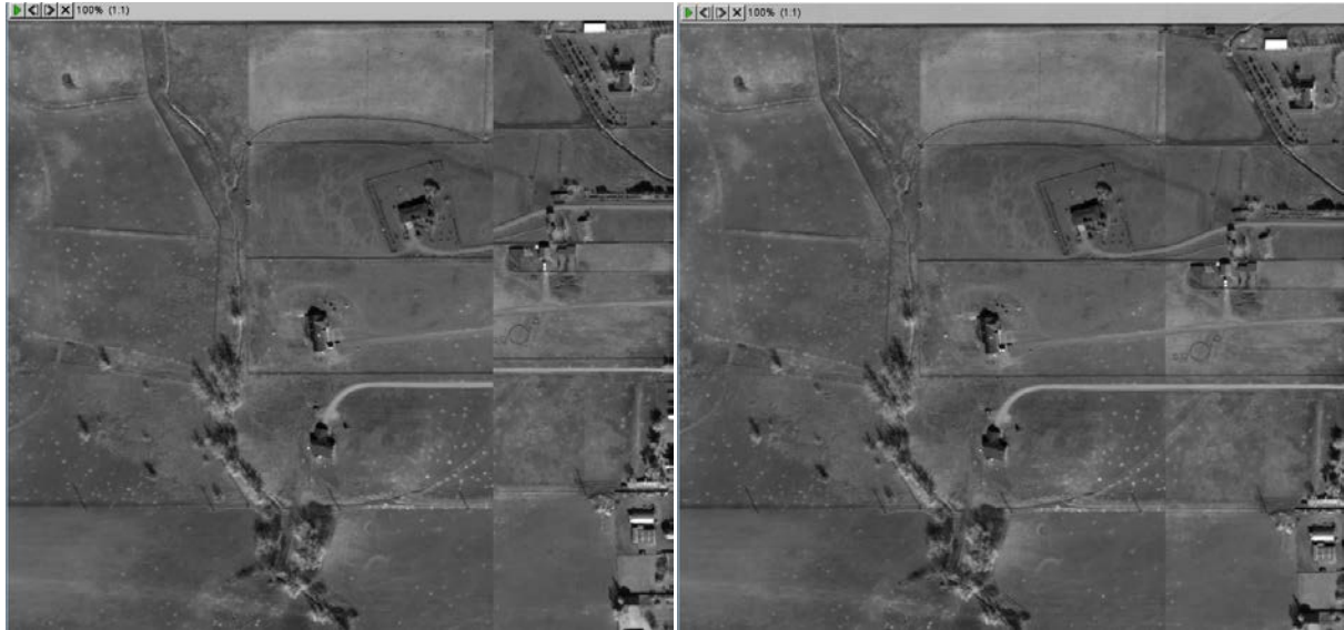
Figure 2. Image registration for change detection analysis. a) View Swipe before image registration. b) View Swipe after image registration.
