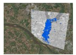
The ENVI SARscape Flood Maping workflow uses one or more pre-flood images, a post flood image, and a DEM to automatically create a classification of flooded areas by comparing the scenes.
