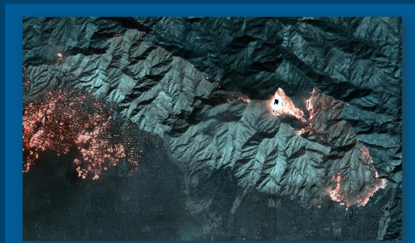
Figure 1: Southern California Wildfire / Eaton (January 2025): WorldView-3 SWIR WorldView-3 SWIR image of the Eaton wildfire, showing active burning fire zones through dense smoke. SWIR not only penetrates smoke and haze, but also reveals high-temperature areas such as active fires and burn scars, enabling fire detection when aerial surveys are limited by smoke, darkness, or wind.
