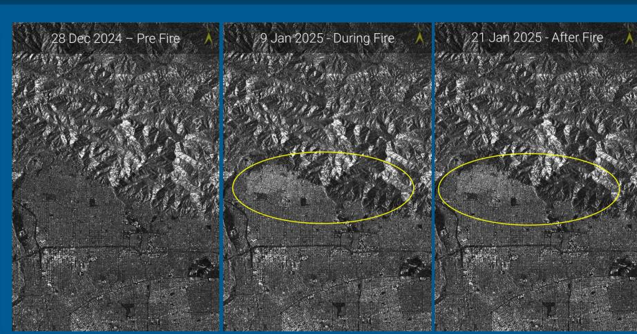
Figure 2: Southern California Wildfires / Eaton (January 2025): SAR Sentinel-1 Time Series (VH) Difference in backscatter mainly because of change in vegetation cover: Following the fire, urban areas appear much brighter and clearly delineate from surroundings, because of now ruined and uncovered building structures as result of disappeared vegetation. Controversially, in the mountain areas, vegetation burnt down as well, but is now exposing bare ground.
